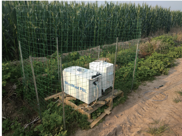
图 1 WindMast PBL 多普勒测风激光雷达 Fig.1 WindMast PBL (Doppler wind lidar)
