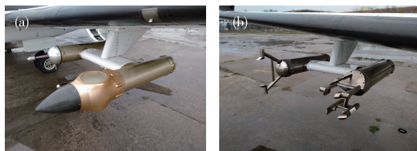
图 1 机载探测设备示意图(a. KPR, b. DMT) Fig.1 Airborne detection equipment (a. KPR, b. DMT)
